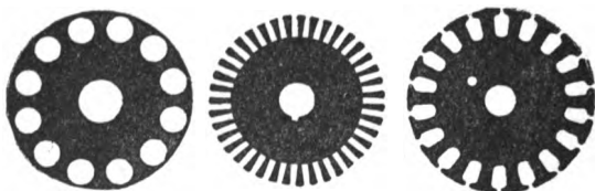
Forms of annealed steel discs used in armature construction
