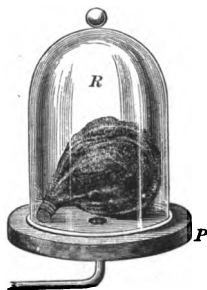
Fig. 45.—Expansion of Air in Vacuous Space.
