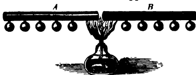
Fig. 60.—Unequal Conduction of Copper and Iron.
