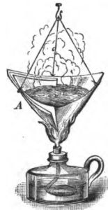
Fig. 64. Water Boiled in a Paper Bag.
