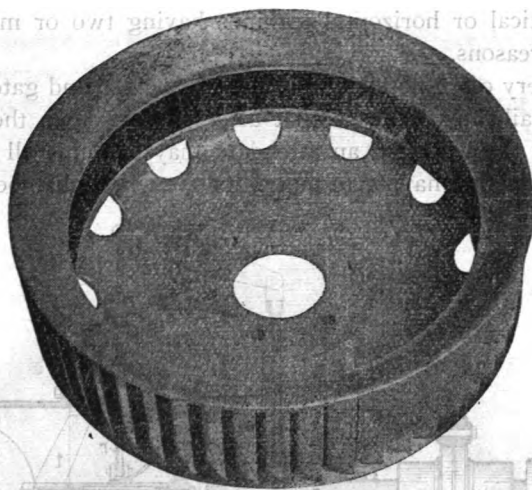
Fig. 153.—Runner of Girard Turbine. Type C, High-Pressure Runner. Platt Iron Works Company (see page 235).
